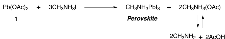
Scheme 1. Proposed formation mechanism of \text{CH}_3\text{NH}_3\text{PbI}_3 from \text{Pb(OAc)}_2 2)
