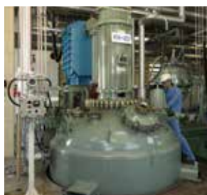
Reactor: 8000 L Glass-lined
