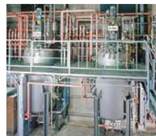
Fermentation Tanks: 2000 L Stainless Steel
