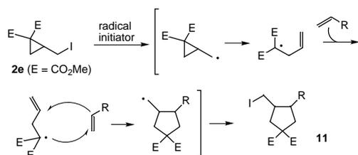
**Scheme 13.** Radical iodine atom transfer [3+2] cycloaddition with iodomethylcyclopropane.
