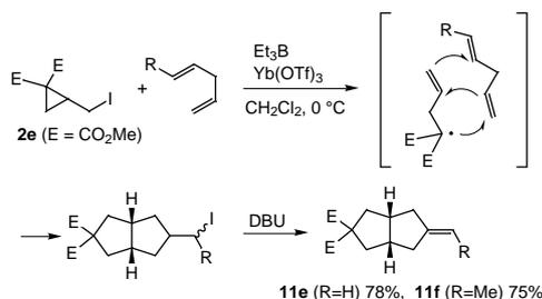
**Scheme 15.** Radical cascade cycloaddition of iodomethylcyclopropane with 1,4-dienes.
