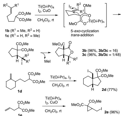
**Scheme 3.**  $\text{Ti}(\text{OR})_4$ -mediated iodocarbocyclization of various alkenylated malonates.
