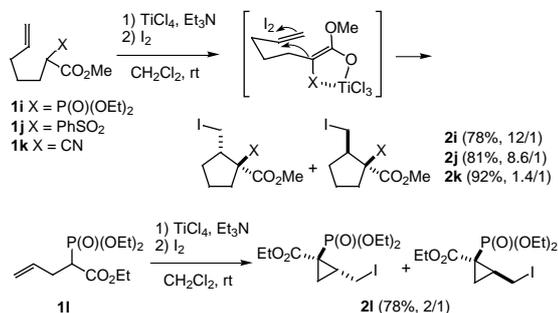
**Scheme 5.**  $\text{TiCl}_4$ -mediated iodocarbocyclization of various alkenylated active methine compounds.
