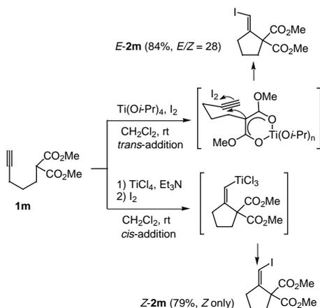
**Scheme 6.** Iodocarbocyclization and intermolecular carbotitanation of alkynylated malonates.
