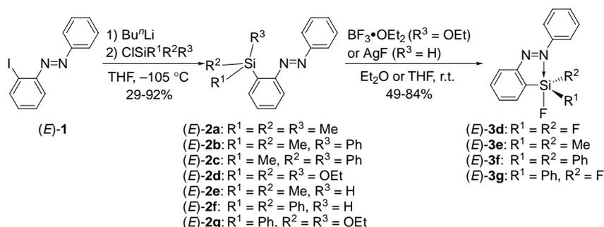
**Figure 2.** Synthesis of pentacoordinated fluorosilanes bearing an azo group.
