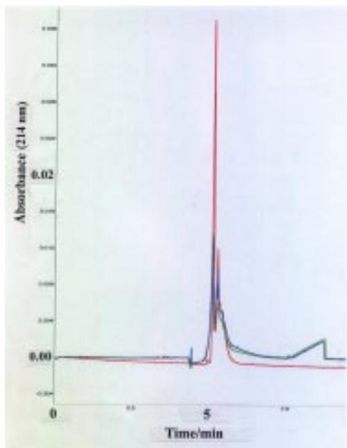
**Fig. 7.** CE profiles of the solutions containing SOD (SOD 3 mg/1ml). red: SOD only. Green and blue: copper(II)/ascorbate solution was added to SOD solution. (green, measured immediately after addition, and blue, at after 60 min.)
