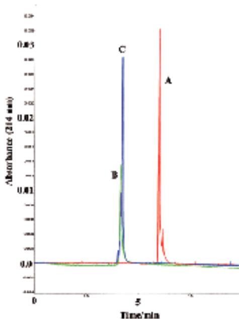
**Figure 6.** CE profiles of the solutions (protein 2 mg/1ml). A: SOD; B: Apo-transferrin, and C; Fe(ida) complex was added to solution B.
